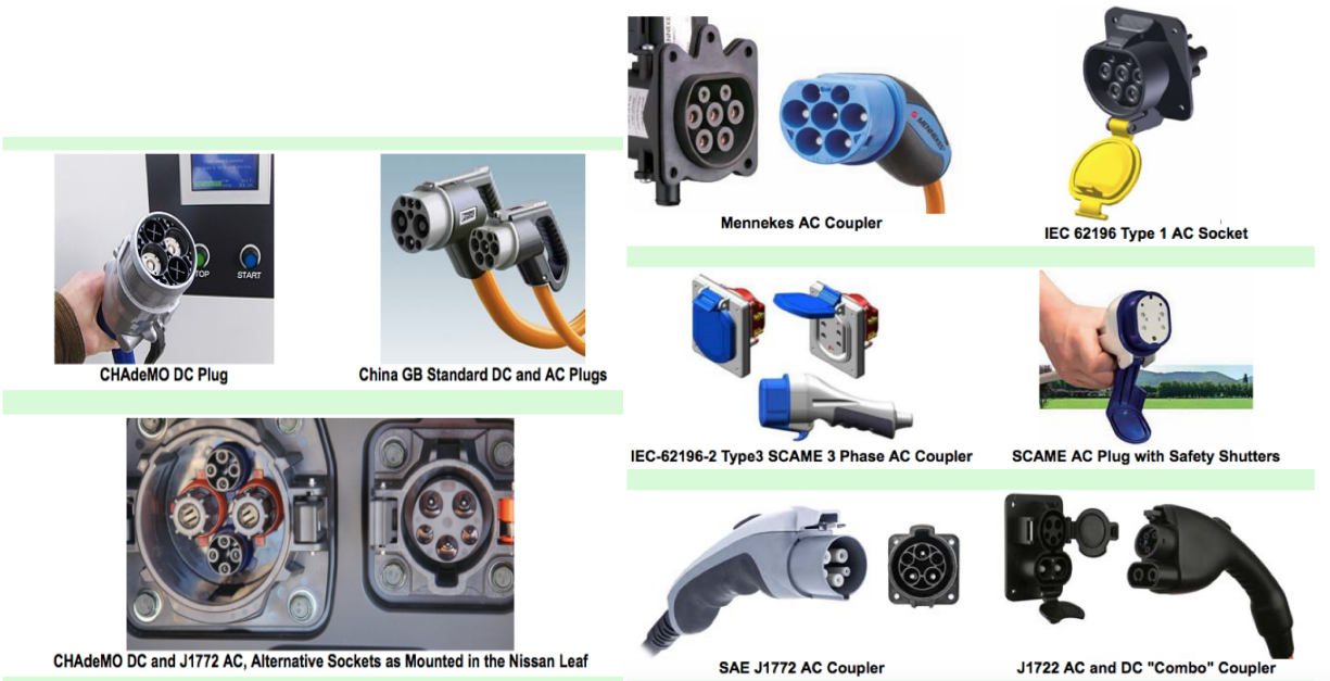
[Fig-15_2] EV Charge Couplers
